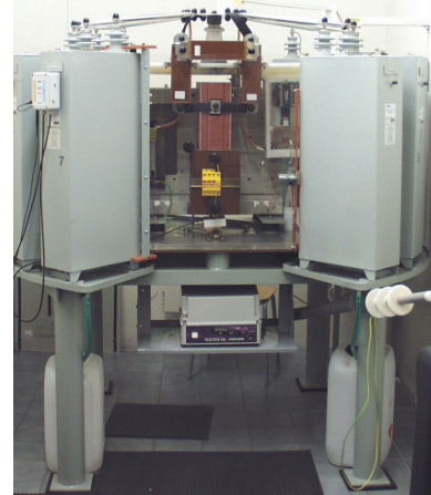
HAKELGUN 240: Testing current pulse generator with the operational capacity up to I_{\text{max}} = 240\text{kA}(8/20)
