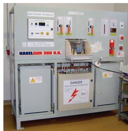
HAKELGUN 200BB: Lightning current generator with the operational capacity I_{\text{imp}} = \text{up to } 210\text{kA}(10/350) .
